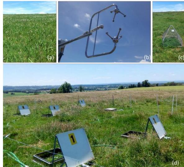
**Fig.1** Field measurements of GHG emissions at Laqueuille site (France). Site (a), flux tower for C fluxes measurements (b), grazing exclosure cage (c) and automatic chambers for N<sub>2</sub>O measurements (d). Photograph credits: F. Ehrhardt, July 2016.
