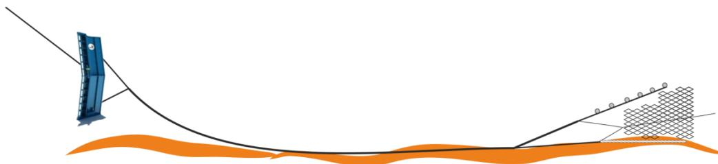
Figure 7.5.2. The use of a) flying/pelagic doors in bottom trawls,
