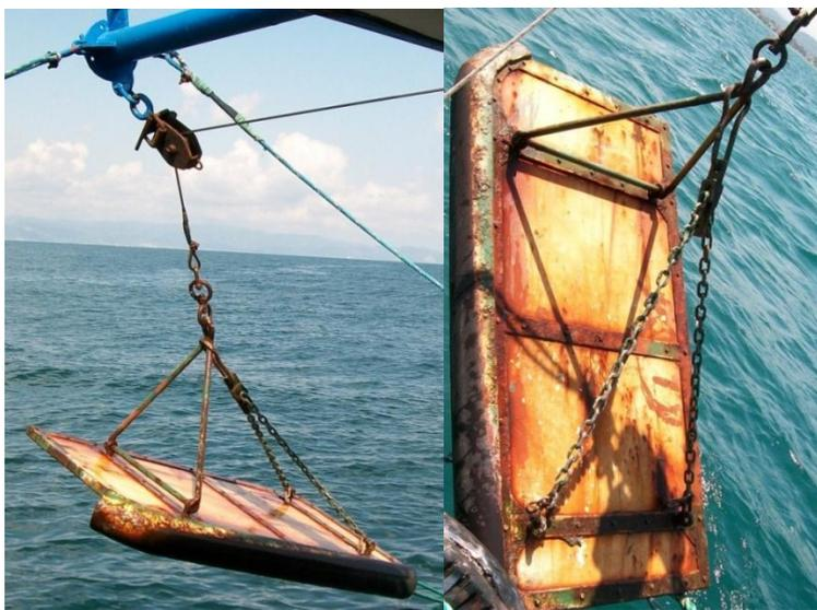
Figure 6.3. A typical rectangular bottom trawl door is using in the SSA
