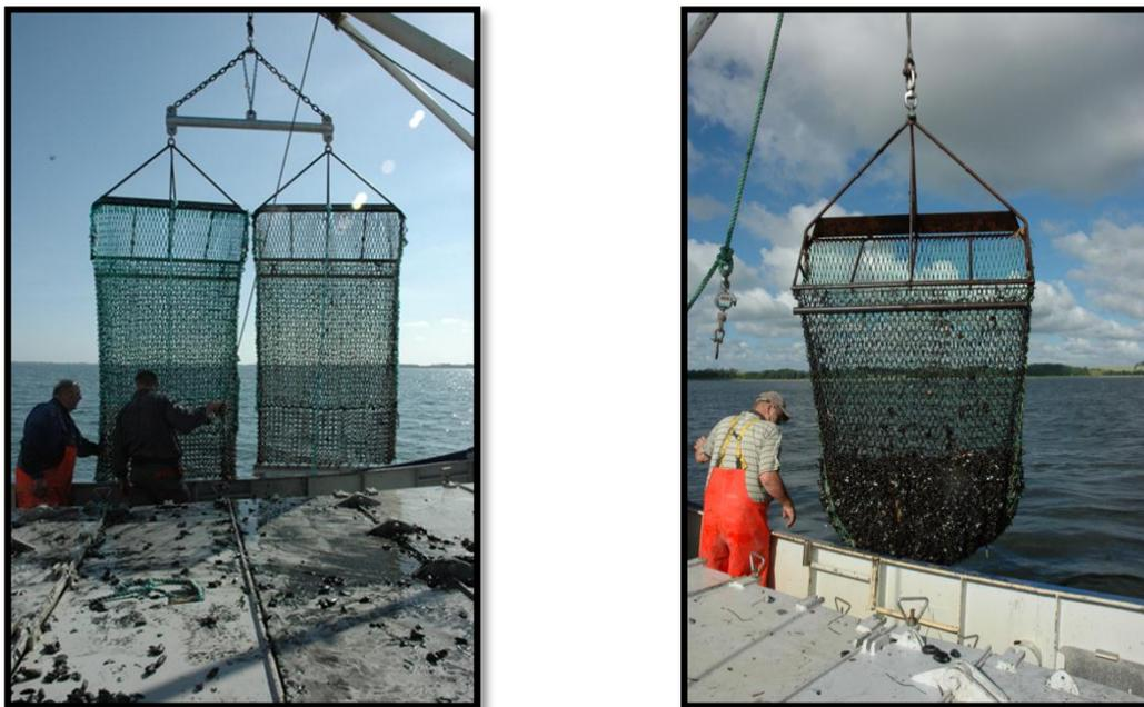
Figure 2.1. Different types of mussel dredges – light at the left and standard heavy at the right hand side.
