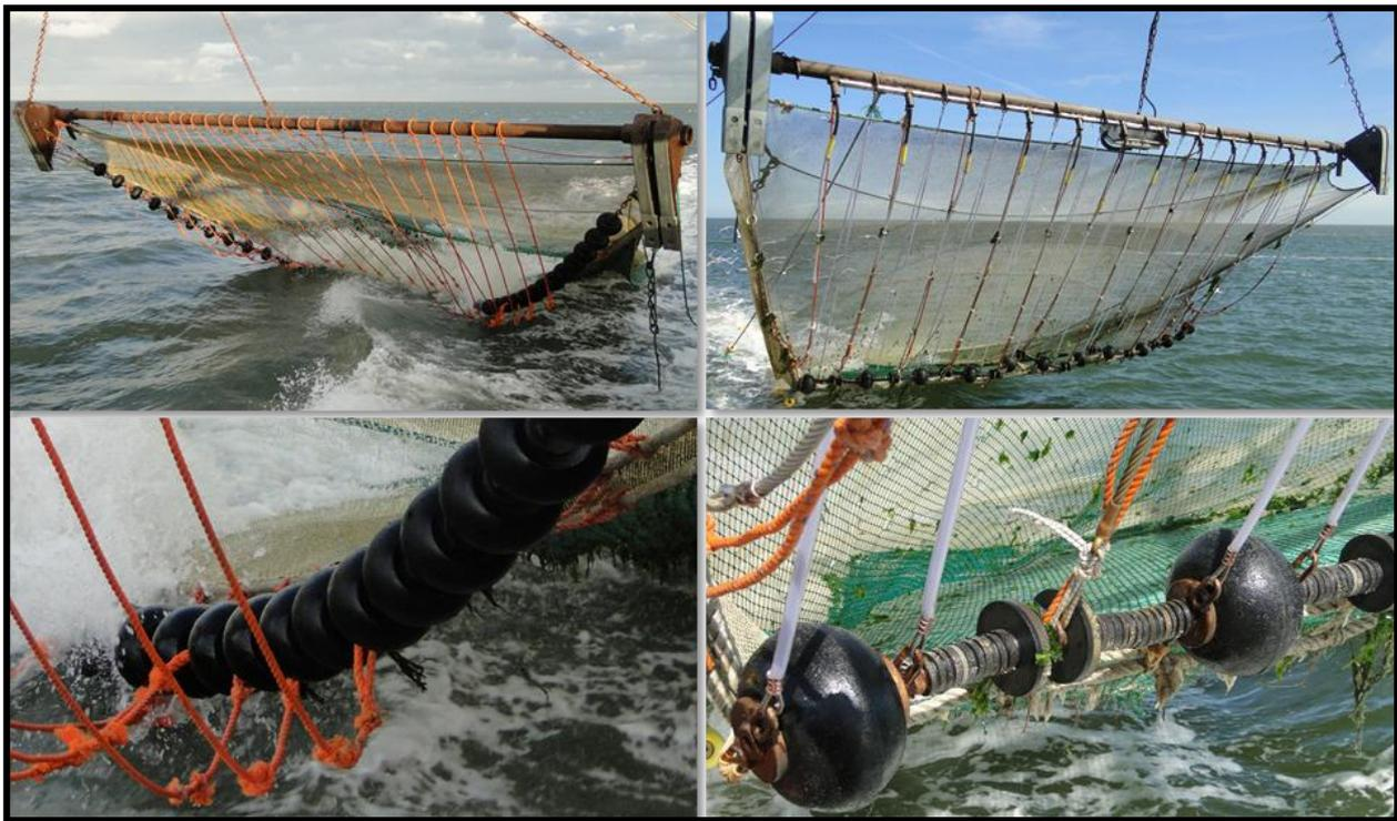
*Fig. 3.5– The two main designs of the shrimp beam trawl. Left: the traditional shrimp trawl with round bobbin rope of 400 kg (and optional beam/groundgear connections). Right: the shrimp pulse trawl with straight bobbin rope of 155 kg and electrodes.*
