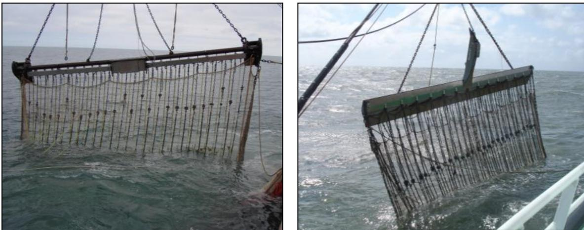
Fig. 3.4– The two main designs of the pulse trawl.
