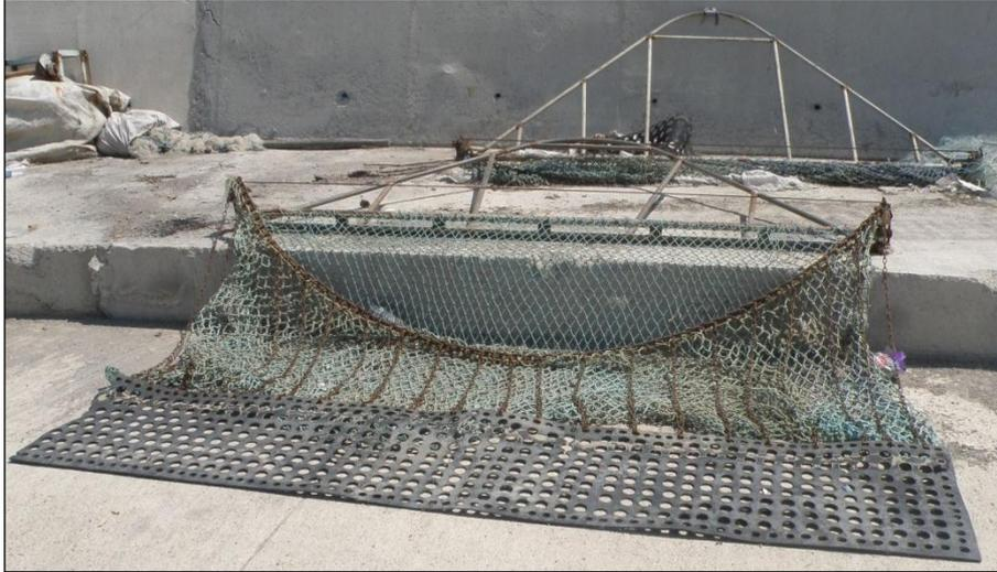
Figure 6.8. There is a perforated plastic/rubber palette attached to the chain on the opening of the gear, in order to mitigate the friction beneath the gear and to provide an easier slipping and also to minimize the gear deformation. Furthermore, to protect the upper panel of the gear, a covering (mantle) was added to the gear produced with a larger mesh size than of the bag and with a coarser thread material.
