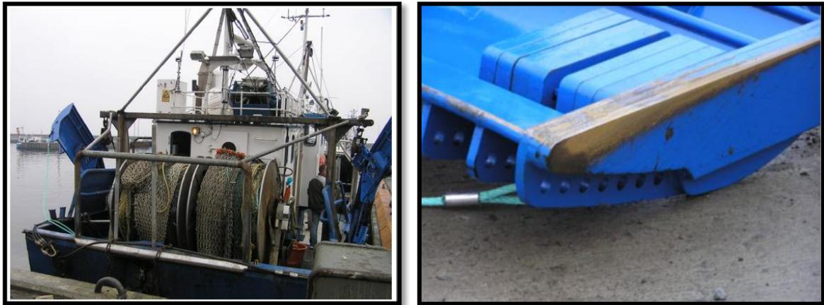
Figure 2.2. Pelagic trawl doors compared to standard trawl doors in demersal cod trawl fishery.
