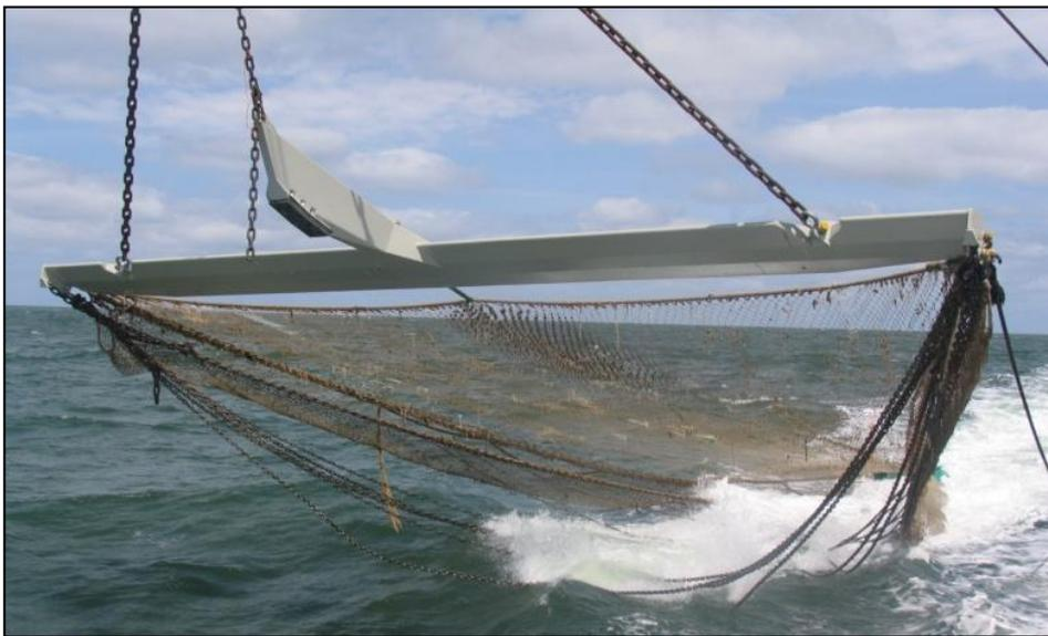
Fig. 3.2- The Sumwing with tickler chains.
