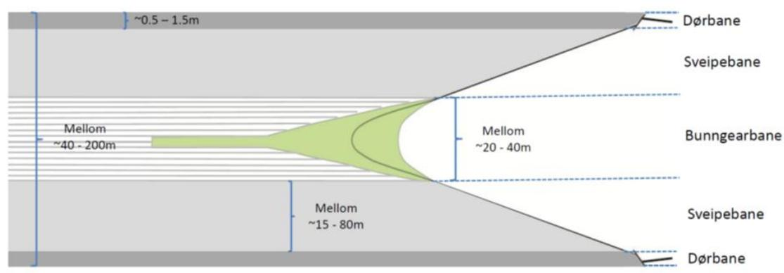
Figure 2. Conceptual footprint from standard otter trawls with three types of sea bed impacts: 1) the track affected by the otter boards ("Dørbane"), 2) the track influenced by the sweeps ("Sveipebane") and 3) the track affected by the trawl itself ("Bunngearbane"). Illustration from Buhl-Mortensen et al. 2013.
