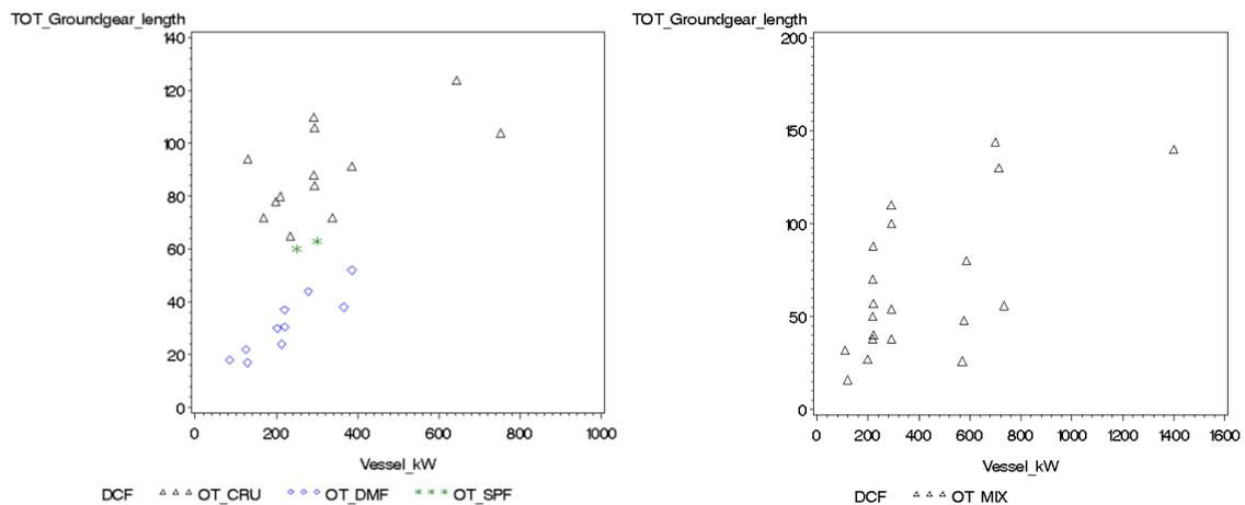
Figure 11. Ground gear length against vessel kW by metier (OT=Otter board trawls, CRU=crustaceans, DMF=demersal fish, SPF=small pelagic fish and MIX=mixed crustaceans and demersal fish).
