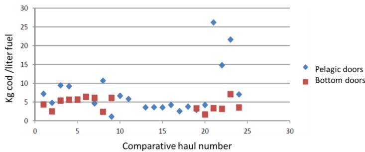
Figure 4. Cod catch weight (kg) per liter fuel consumption for the same trawl and sweep lengths fished with pelagic doors (blue diamonds) and bottom doors (red squares) from the same vessel, but on different trips (Gemba, 2011).
