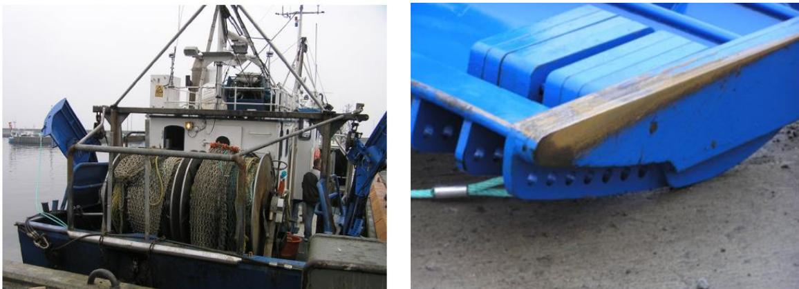
Figure 3. Pelagic trawl doors compared to standard trawl doors in demersal cod trawl fishery.
