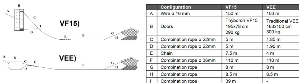
Figure 21. Main details of the gear rigging adopted during the sea trials. Configurations with the Thyboron type VF15 (VF15) and with the traditional VEE door (VEE).
