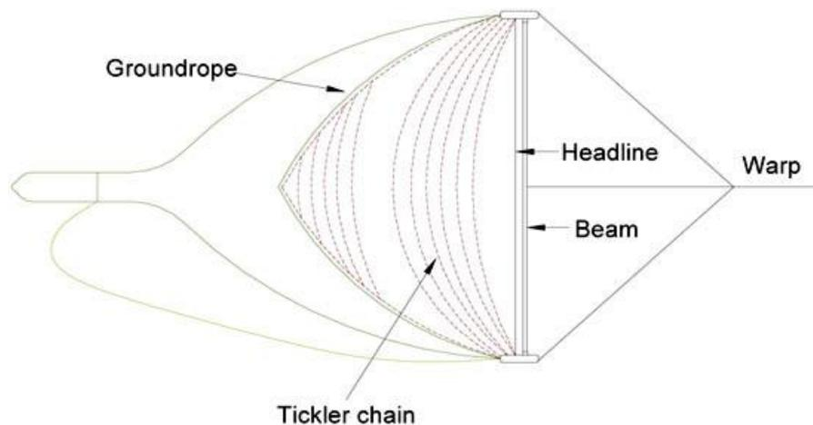
**Figure 5.5.** Drawing of beam trawl with warp, beam, shoes, tickler chains and ground gear (illustration from FAO Fisheries Technical Paper 472)
