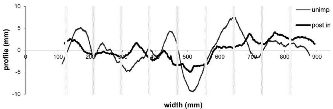
**Figure 5.9.** Profile of un-impacted and post impacted seabed measured using the laser stripe profiler. The vertical lines represent the possible position of the scallop dredge teeth and coincide with local minima of the post impact profile (O'Neill et al 2013).
