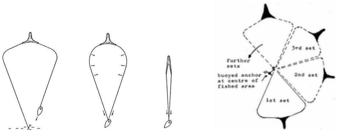
**Figure 5.10.** Left: Illustration of three steps in an individual anchored seine haul, Right: the combined gear footprint of a series of four seine hauls (illustration from <http://www.fao.org/fishery/geartype/203/en>)
