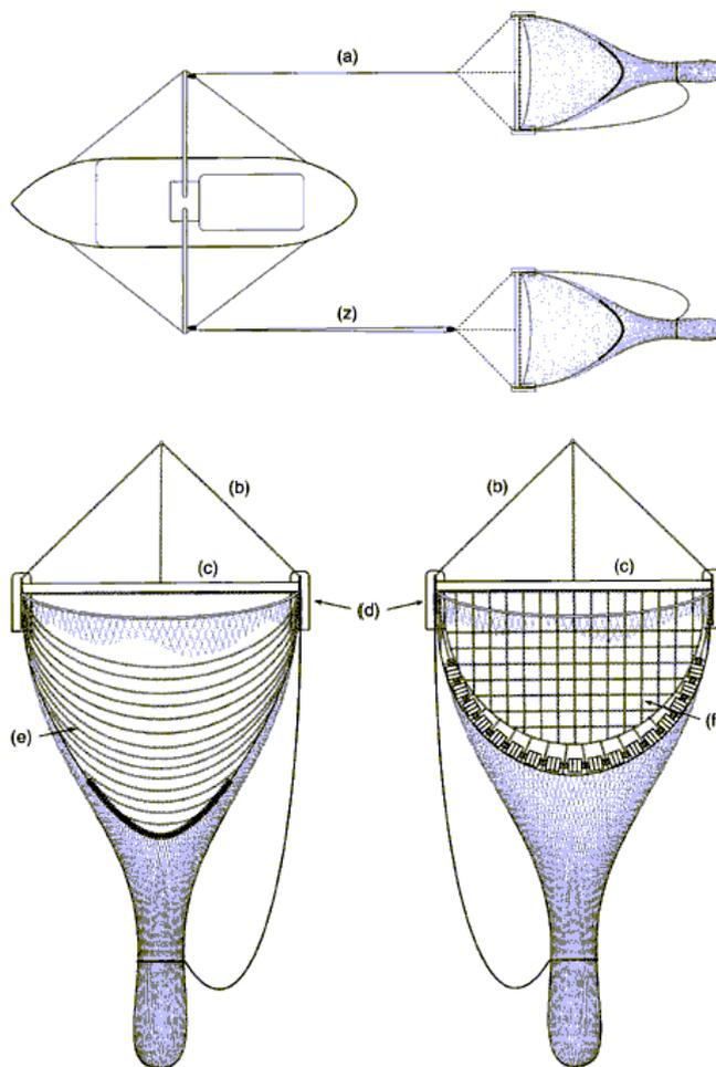
Figure 7. Twin beam trawls
